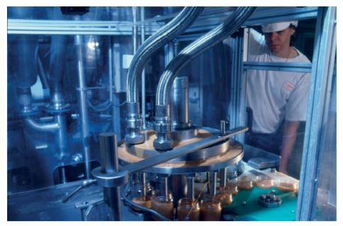
PTFE has a number of special characteristics, giving the hoses a very wide application field within the various branches of industry. Target applications are in the chemical, pharmaceutical and food industries. These industries employ the hoses for steam, air, oil, chemicals, acids, alcohols, solvents, refrigerants, gases, foodstuffs, cosmetics, etc. as a cable protection sleeve or as a level gauge tube.
