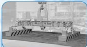
PH 2/7: Beam with electromagnets for horizontal handling
