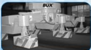
Beam with spring suspended electro-permanent magnets for handling large steel plates
