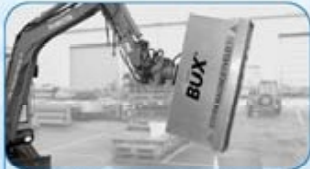
Permanent, deep field, hydraulically operated magnet fitted to mini excavator for cleaning yards
