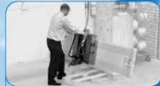
Pneumatically operated permanent magnets for lifting and turning packed radiator panels
