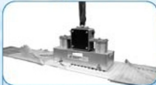
Pneumatically operated permanent magnet for lifting radiator panels
