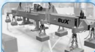
Telescopic, motor driven beam with electro-permanent magnets for handling large steel plates
