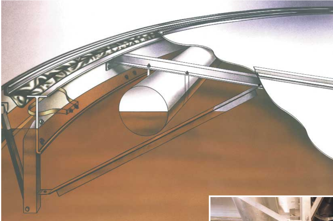
Primary stainless steel shoe seal
