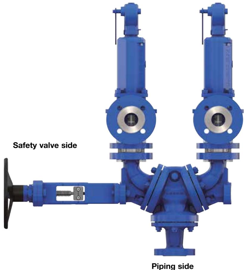
Change-over valves are used to connect two safety valves with a pipe connection to a pressure system, in order to increase operational availability. One safety valve is in operation and one safety valve is on standby.
